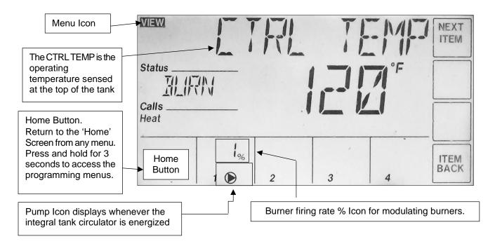
The **View Menu** is the default display (home screen) of the EOS control system. The View Menu displays general information about the water heater's operation and status. The default display includes a Burner Firing Rate % Icon, a Pump Icon that is visible whenever the integral tank circulator is energized and Failure Messages if the unit is in an alarm or error condition.
