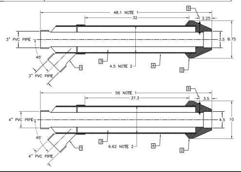
**Note:** Dimension may be shortened to a minimum of 12". Inner pipe (item 3) must remain 10" longer than the outer pipe (item 4). Cut pipe ends square and solvent cement as outlined in the System 636 installation manual.
