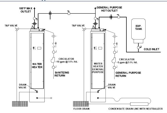
Figure 4-5: Configuration for Booster Heater Application
