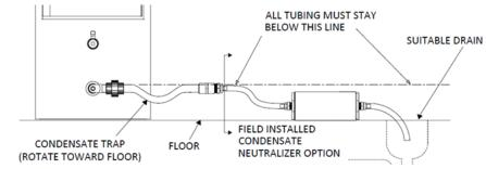
Figure 5-2: Condensate Trap with Optional Condensate Neutralizer on Same Level
