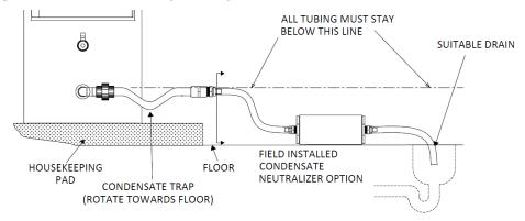
Figure 5-3: Condensate Trap with Optional Condensate Neutralizer Located Below Unit
