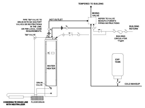
Figure 4-1: Single Water Piping
