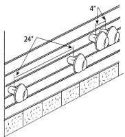
Figure 8-3: Sidewall Termination for Multiple Horizontal Concentric Vent
