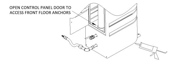
**Figure 16-1: Front Floor Anchor Location**
