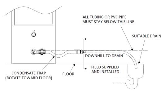
Figure 5-1: Condensate Trap without Optional Condensate Neutralizer
