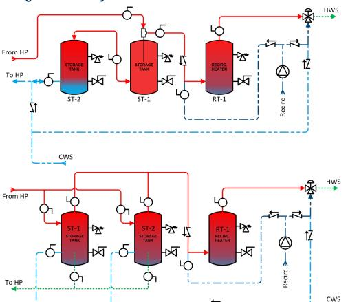
**Single-pass** heat pump example configuration with recirculation
