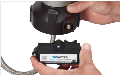
5. Press the activation module onto the sensor.
