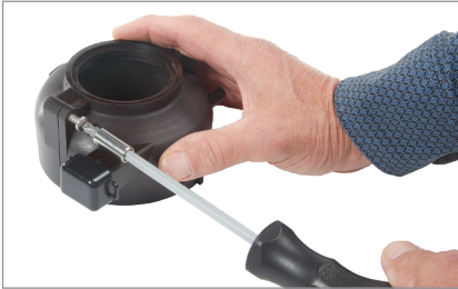
1. Remove the bolts from the flood sensor.
