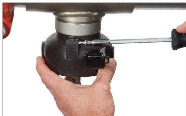
3. Insert the bolts and tighten.
