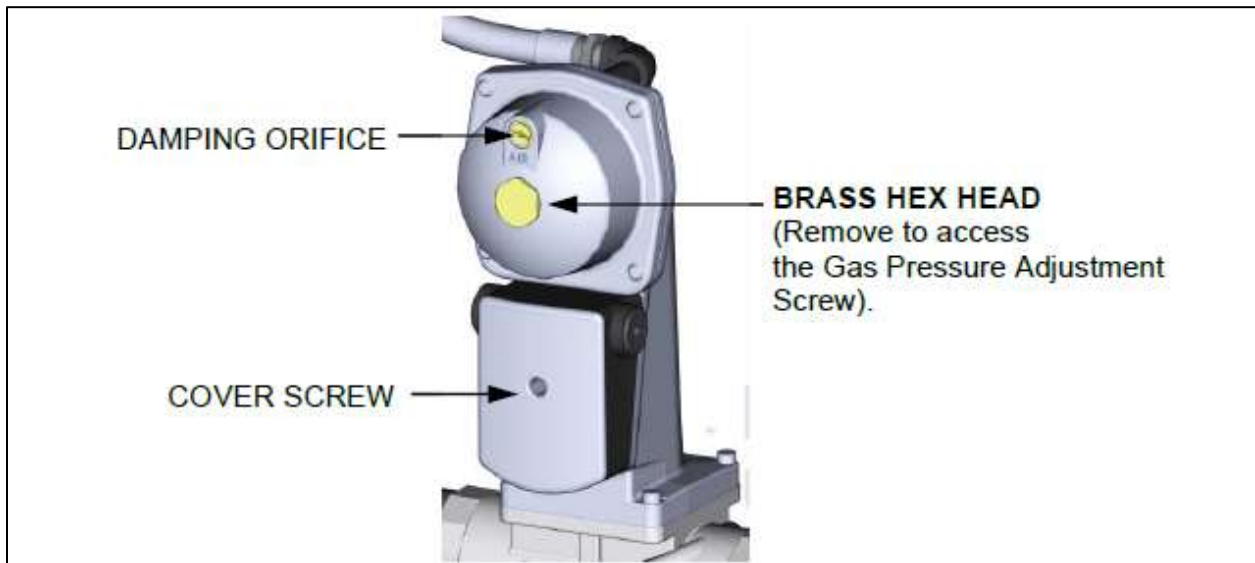
Figure 10-3: SSOV Actuator with Gas Pressure Adjustment (SKP25)
