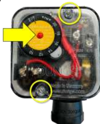
Figure 6-3: High Gas Pressure Switch
