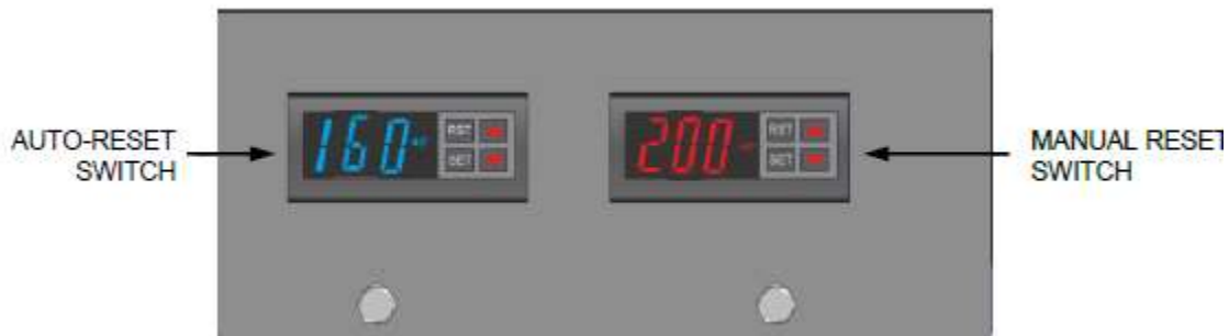
Figure 5-8: Over-Temperature Limit Switches
