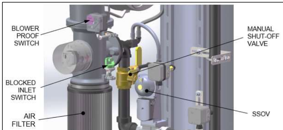
Figure 6-7: Blower Proof & Blocked Inlet Switch Locations
