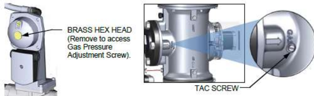
Figure 5-4: Gas Pressure Adjustment Screw and TAC Screw Location
