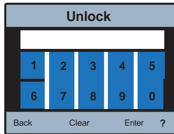
To unlock the control select the **UNLOCK** icon from within the “Programming” menu.
