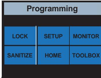
Select the **SETUP** icon from within the “Programming” menu to access the “Setup” menu shown below.
