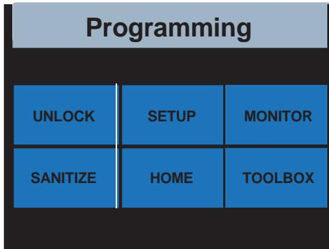
3. On the Programming Menu, touch the **UNLOCK** icon. The Unlock function screen will appear and you will be prompted to enter the passcode:
