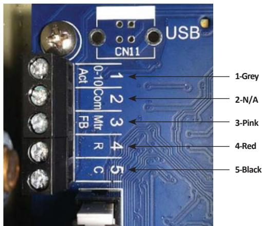
3. Locate the Actuator Cable. Remove the Actuator Cable from the control box and stand supports. If needed, snip cable ties making sure not to damage any other wires when removing the cable ties.
