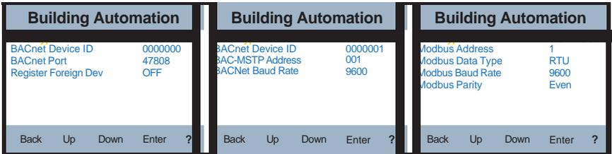
Each of the settings can be adjusted by depressing the **Up** and **Down** icons to highlight the setting of interest and depressing the **Enter** icon to adjust the setting.
