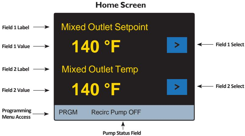
As shown in the screen shot above, there are two fields viewable within the "Home" screen. For instance, the Label (item) and Value for Field 1 and Field 2 shown in the Home screen view above are:
