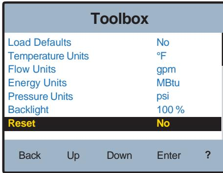
6. On the “Toolbox” menu use the **Down** icon to highlight “Reset” as shown above then press **Enter**. This will access the “Reset” menu shown below.
