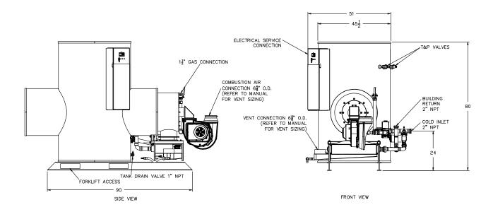
Recommended Service Clearance: 18" from all sides, 12" from the top. Consult factory for heat exchanger pull space requirements. Minimum Clearances: 6" from all sides and top, 24" from the front.
