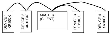
Figure 5 Wiring is not correct. Not a daisy chain and the master is not at an end.
