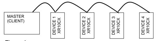
Figure 4 Correctly wired RS-485 Daisy Chain
