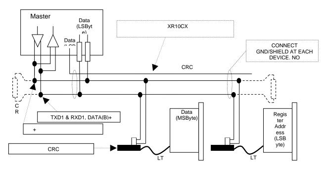
Figure 3 Wiring of a typical Modbus RTU network with XR10CX devices
