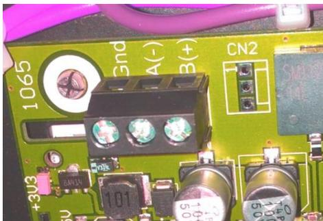
The RS-485 PORT: Both MODBUS RTU and BACNET MSTP connect to this port, selecting the protocol is done in the settings on the display.
