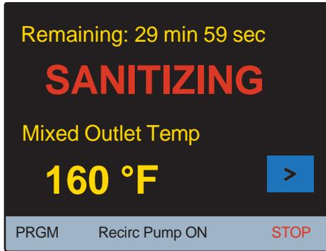
9. After Sanitization Mode has completed (user selected run time has elapsed), the DigiTemp™ will go into a Cool Down Mode to return to the Mixed Outlet temperature prior to sanitizing.
