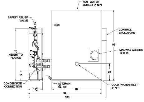
Completed piping assembly is factory fit between the exchanger and tank and is separated at unions for shipping.
