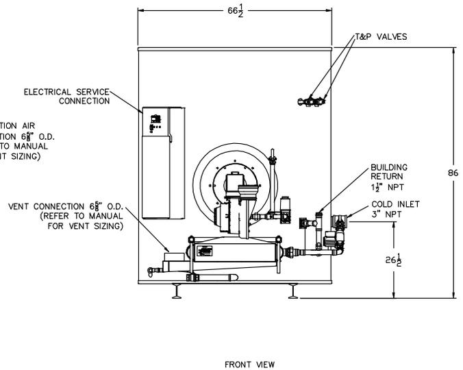
Recommended Service Clearance: 18" from all sides, 12" from the top. Consult factory for heat exchanger pull space requirements.
