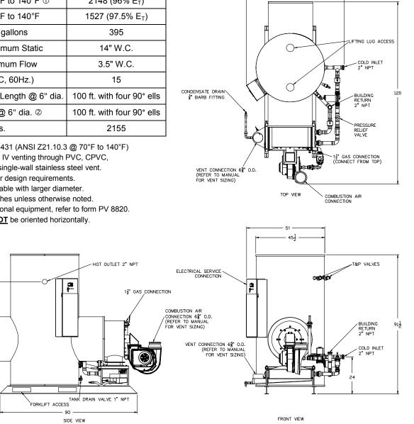
Recommended Service Clearance: 18" from all sides, 12" from the top. Consult factory for heat exchanger pull space requirements. Minimum Clearances: 6" from all sides and top, 24" from the front.
