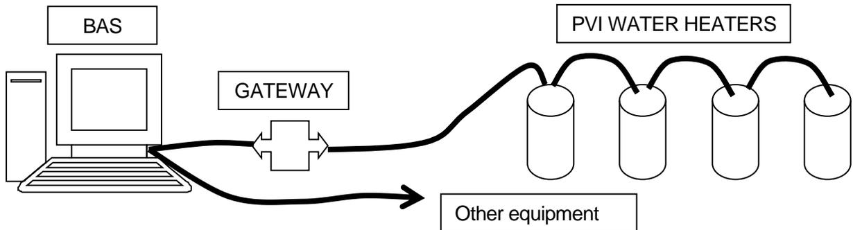
Building Automation System (BAS) connecting to a PVI gateway. This can provide interface to BACNET MSTP, BACNET IP, LONWORKS, and MODBUS TCP.
