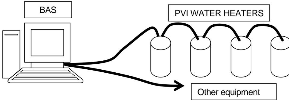
Building Automation System (BAS) connecting directly to water heaters using MODBUS RTU twisted pair wire. (Wiring is RS-485 physical layer.)
