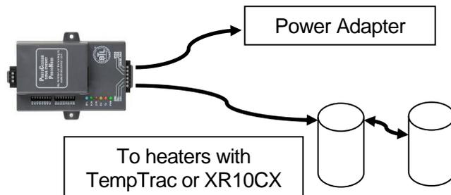
Connection of ProtoNode will be from the 6 pin connector pins 2/3 to the +/1 on the MODBUS adapter ([Return to GETTING STARTED](#))
