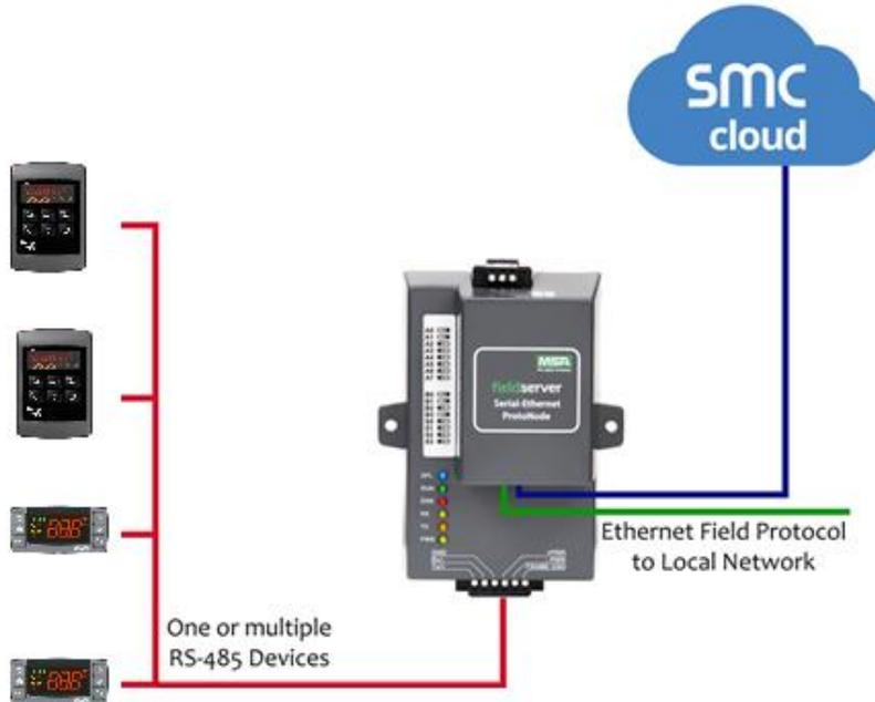
Once configuration is complete, and the interface method is BACNET IP, the connection of the BACNET IP network will be at the Ethernet port of the ProtoNode Gateway.
