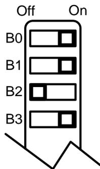
When setting DIP switches, ensure power to the ProtoNode is OFF.
