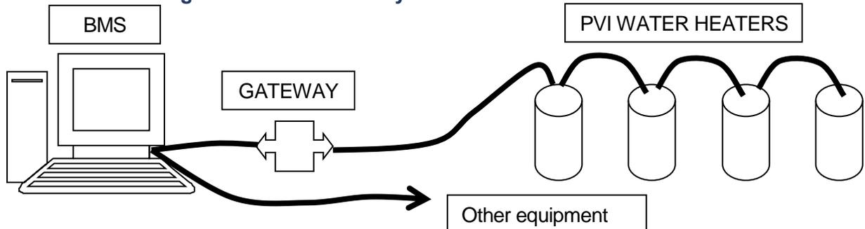
Building Management System (BMS) connecting to a PVI gateway. This can provide interface to BACNET MSTP, BACNET IP, and MODBUS TCP. (Wiring from gateway to heaters is RS-485 physical layer. Wiring from BMS to gateway will be RS-485 for BACNET MSTP, and Ethernet for BACNET IP or MODBUS TCP)
