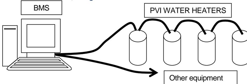
Building Management System (BMS) connecting directly to water heaters using MODBUS RTU twisted pair wire. (Wiring is RS-485 physical layer.)
