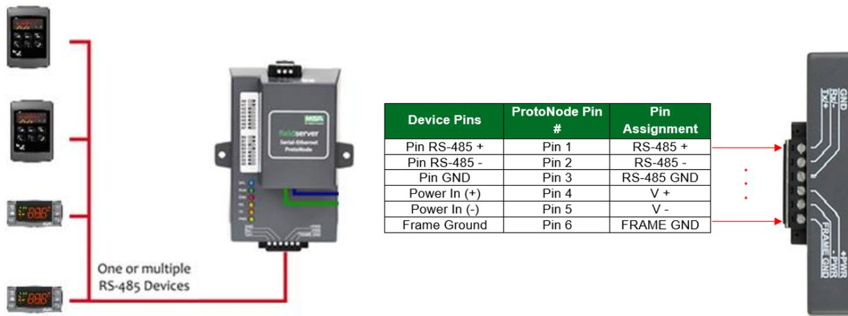
For details of this port on the ProtoNode Gateway see the [ProtoNode S1 Port](#) section. This will show the optional biasing jumpers and the optional termination resistor jumper.
