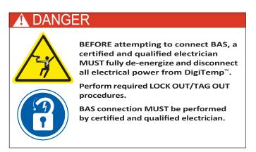
After completely de-energizing and disconnecting all power from DigiTemp™ and performing required LOCK OUT/TAG OUT, carefully open the DigiTemp™ control module by releasing latches to reveal BACnet® and Modbus® hook up terminals.
