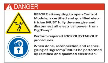
Once de-energized and disconnected, the display will become inactive and the control box can be opened.
