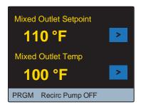
From within the "Programming" menu (shown below) only the HOME and UNLOCK icons are active until the control is in the unlocked state. Note: After 60 seconds of inactivity the control automatically locks and returns to the home screen.
