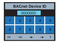
To adjust the ID depress the Del key 7 times and enter an ID appropriate for the remainder of the BAS system and press OK. Similarly, enter an appropriate "BACnet Port." To change "Register Foreign Dev" to "ON" scroll down to "Register Foreign Dev" using the Downicons and select Enter. The "Register Foreign Dev" setting adjustment screen is shown in the "OFF" state below.
