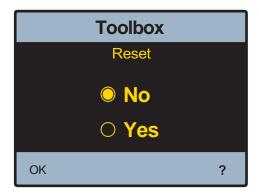
Press the OYes and then OK and the control will reset and begin a start up sequence.
