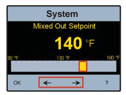
4. Select and set the safe, appropriate and desired outlet water temperature for your users, application and facility by using the slider icor or by touching the right or left arrows until the selected temperature is displayed.
