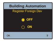
To toggle from "OFF" to "ON" press on the icon next to the "ON" setting to change icon to indicating that this state is what is selected. Press icon to save this setting and return to the "Building Automation" menu shown below with "Register Foreign Dev" set to "ON". Note the additional setting available with the "Register Foreign Dev" set to "ON."
