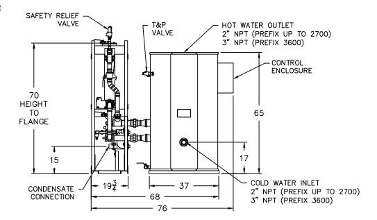
Completed piping assembly is factory fit between the exchanger and tank and is separated at unions for shipping. Tank and heat exchanger ship separately for field connection to piping assembly.
