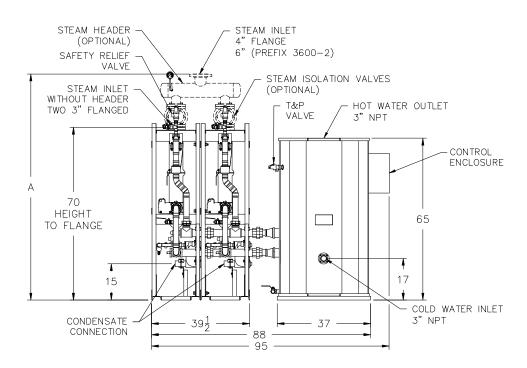
Completed piping assembly is factory fit between the exchanger and tank and is separated at unions for shipping. Tank and heat exchanger ship separately for field connection to piping assembly.
